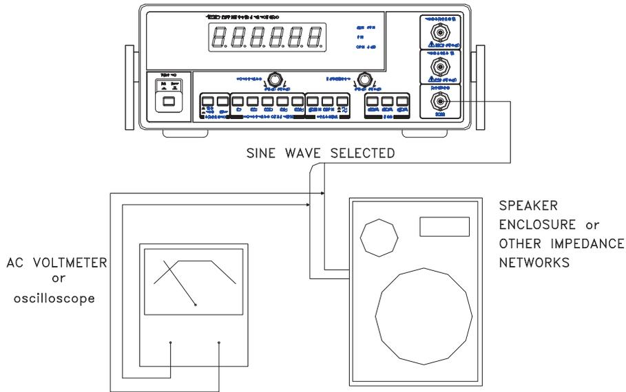
**B. Equivalent Circuit Of Test Set-Up**
