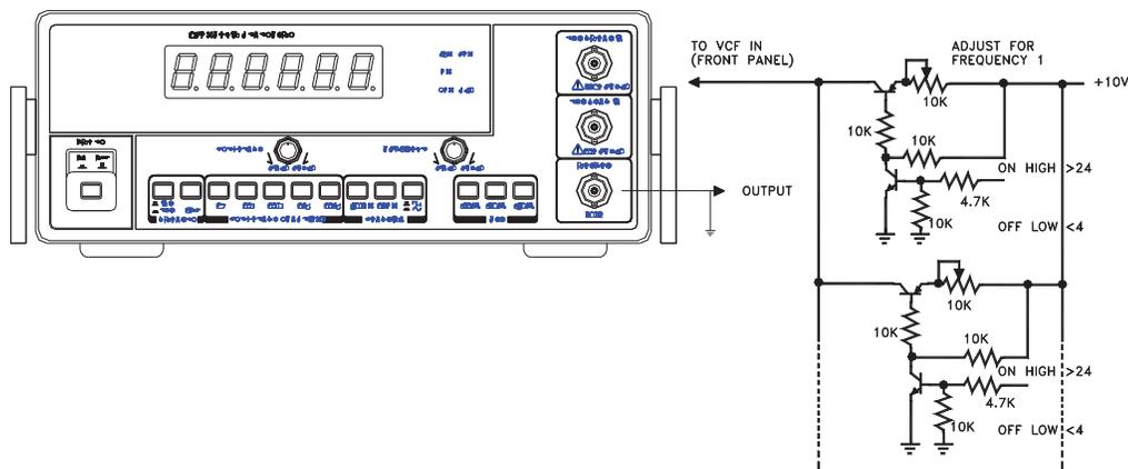
FIG 9. DIGITALLY PROGRAMMED FREQUENCY SELECTION
